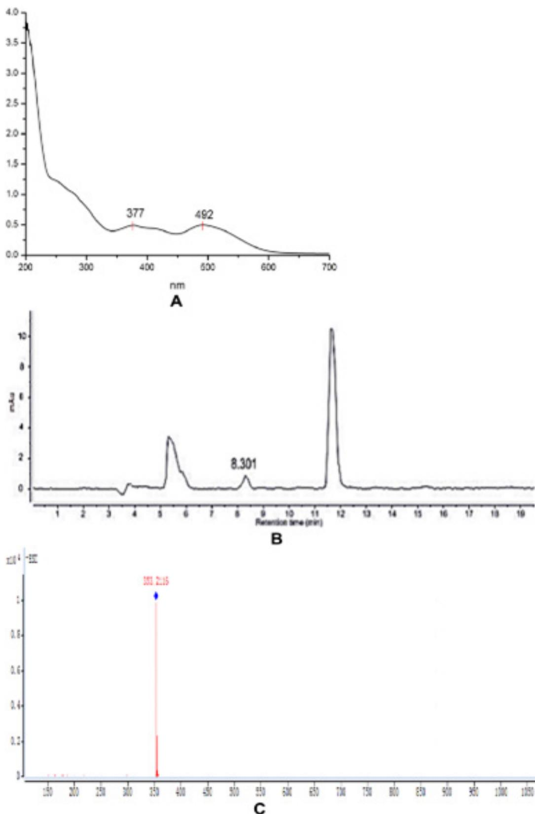
Figure 3. (A) UV-vis absorbance of *Monascus* pigments, (B) HPLC chromatogram of the target pigment, and (C) UPLC-Q-TOF-MS spectrum of the purified pigment from *Monascus*; first order mass spectrum of the target pigment ( $m/z$ ).
