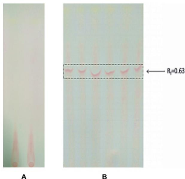
Figure 2. Thin-layer chromatogram of dark red pigments obtained by silica gel column chromatography.
